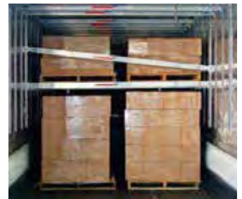
Cargo being restrained by the LIFT-A-DECK System beams.
